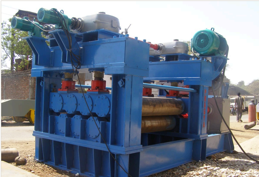
PLATE LEVELER Thickness 0.13-152 mm
