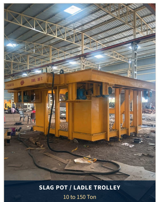
TROLLEY WITH TILTER 0-90° Hydraulic Tilting
